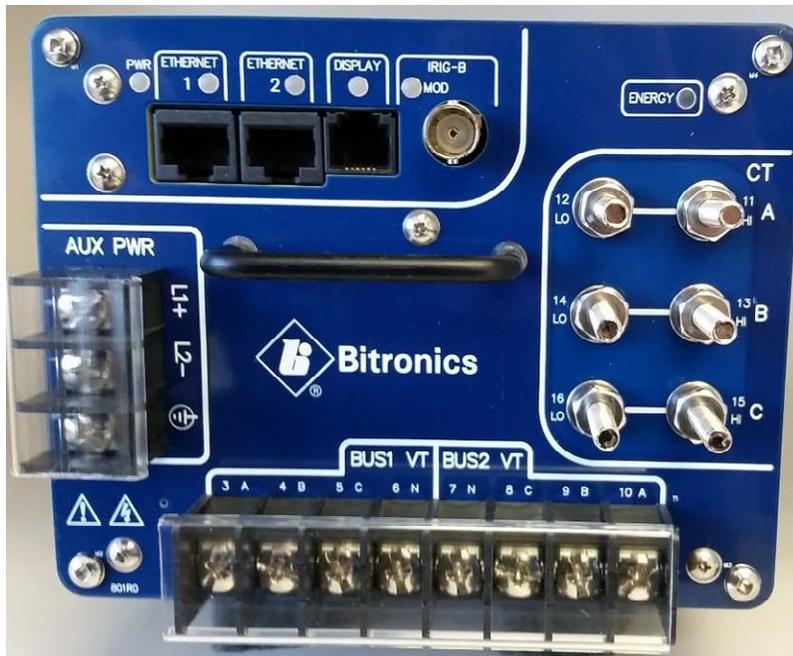
**Figure 3B – PPX II Connection View with Options in Standard chassis for Display port, IRIG-B port, Energy Pulse LED**
