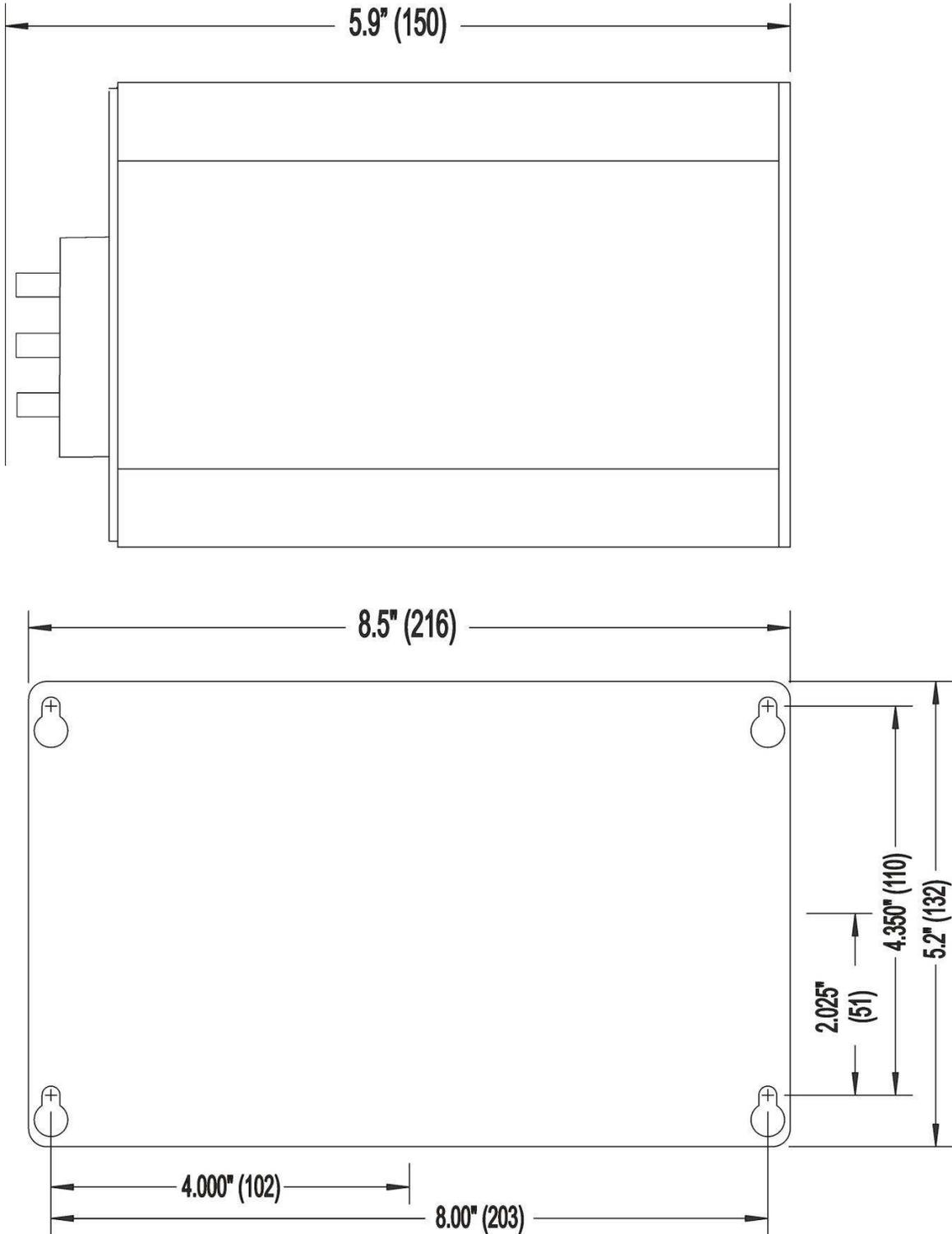
**Figure 4B – Mounting and Overall Dimensions PPX II in Extended Chassis** (back panel may vary as a result of options ordered)
