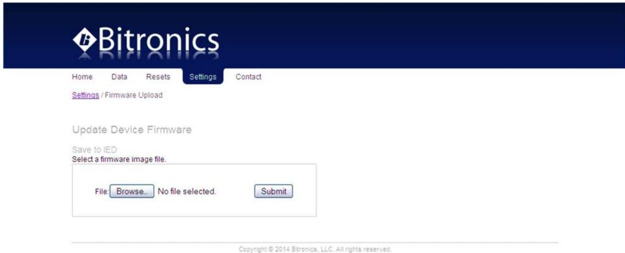
**Figure 7 – Bitronics PPX II Firmware Upload Page**
