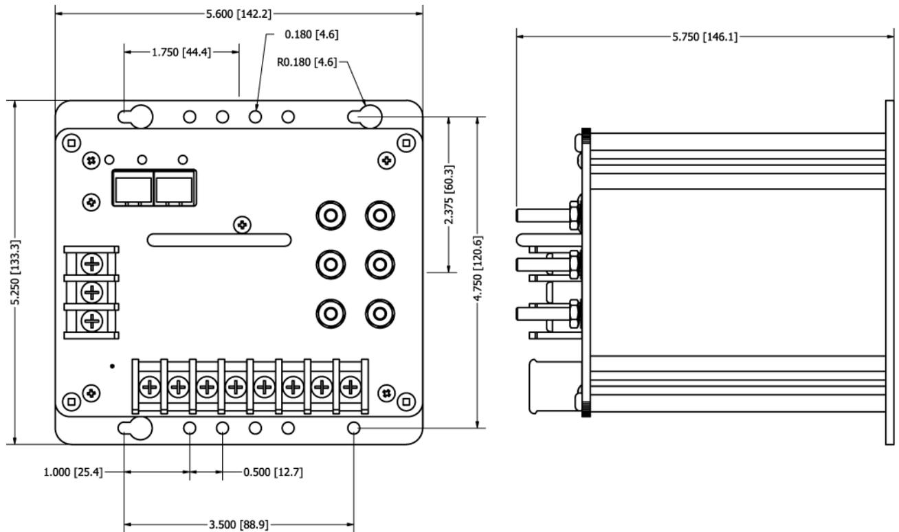
**Figure 4A - Mounting and Overall Dimensions PPX II in Standard Chassis**
