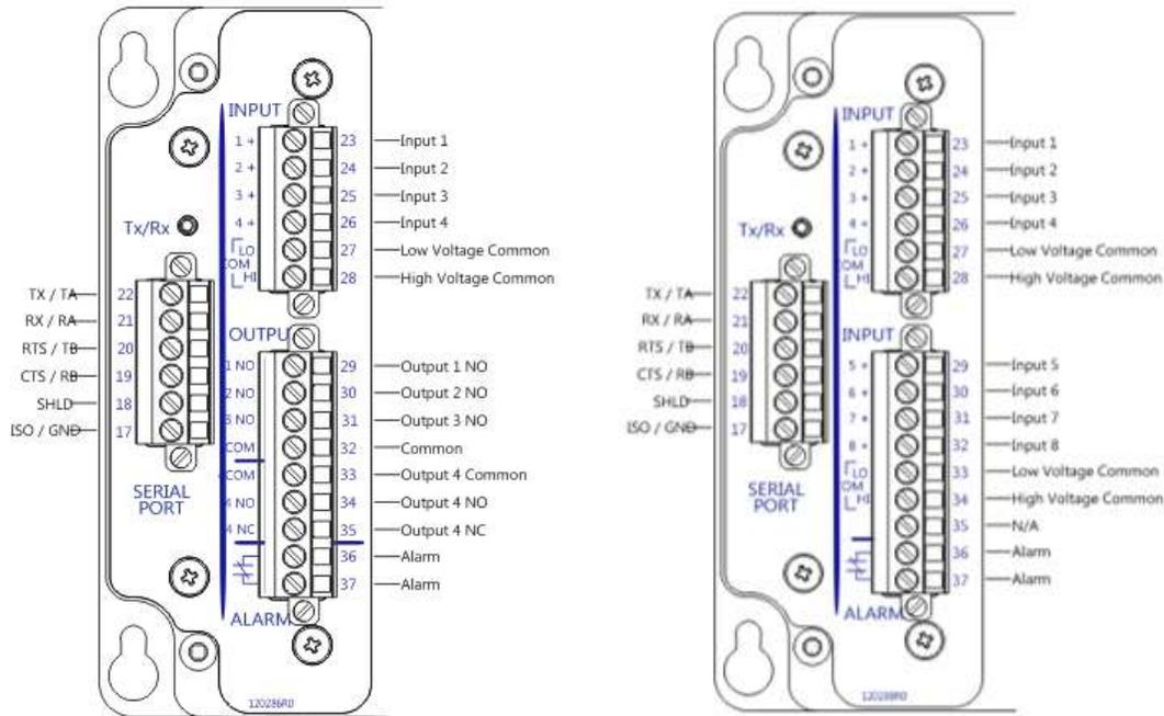
**Figure 2 - Wiring Terminal Assignments for Input and Output Options**
