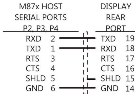
The rear port of the D650 Display and the Host port of the M87x must be set to RS-232, matching Baud rates and parity, and Display protocol.
