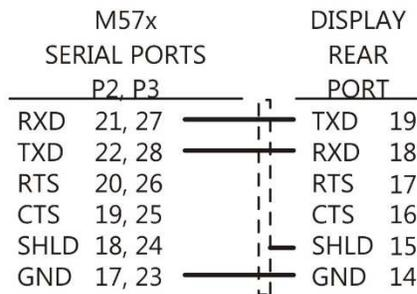
The rear port of the D650 Display and the port of the M57x must be set to RS-232, matching Baud rates and parity, and Display protocol.
