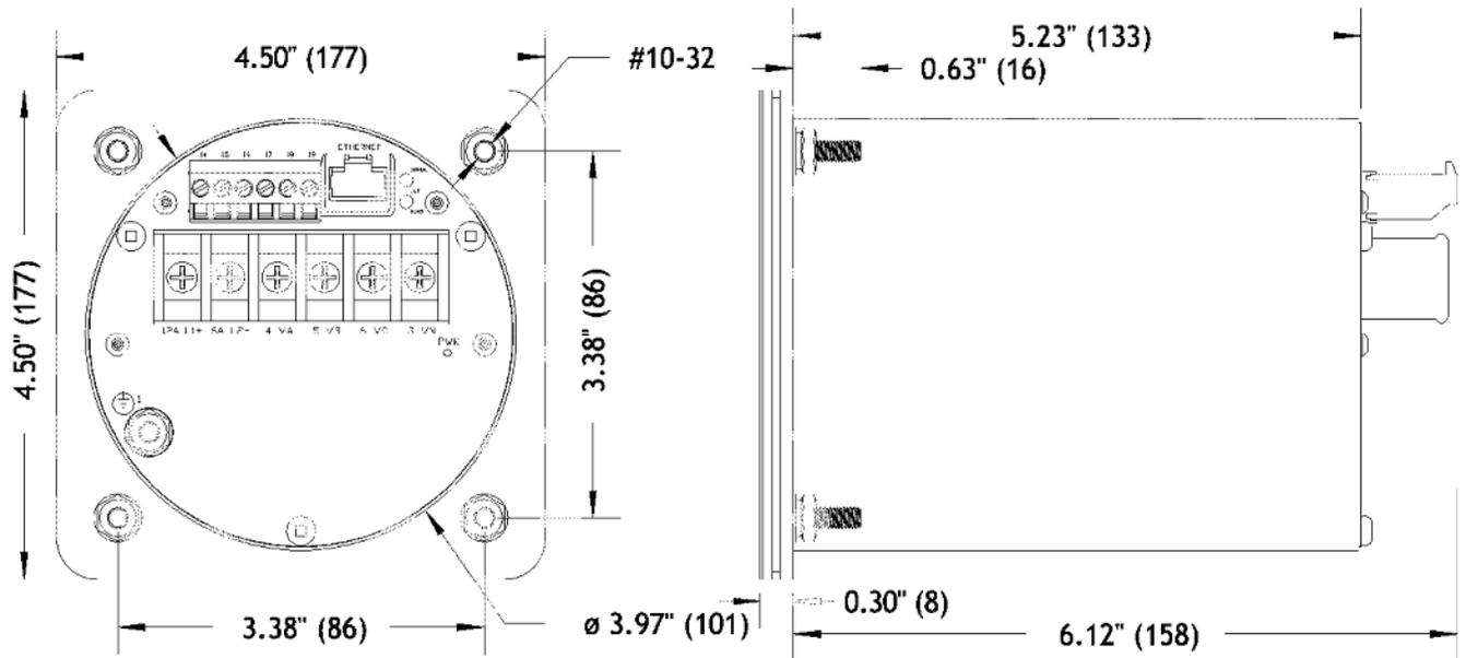
**Figure 2 - Mounting and Overall Dimensions D650**
