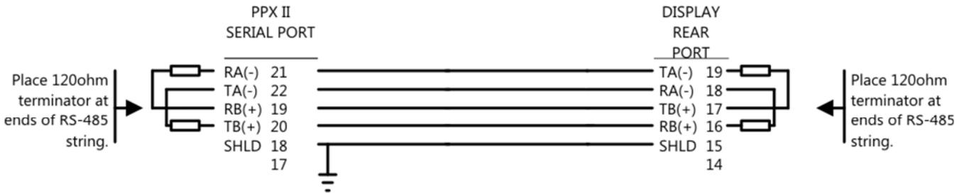
The rear port of the D650 and the serial port of the PPX II must be set to RS-485, matching Baud rates and parity, and Display protocol.
