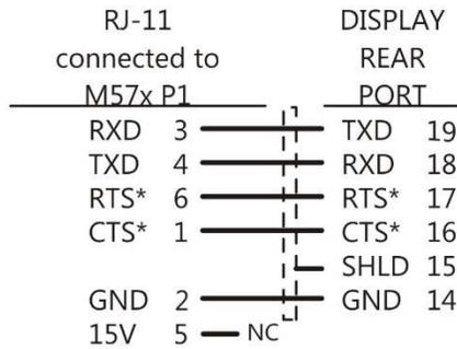
\*6 conductor RJ11 flat cable - RTS & CTS are not required for D650 display operation. Otherwise, 4 conductor RJ11 flat cable will suffice for display operation.
