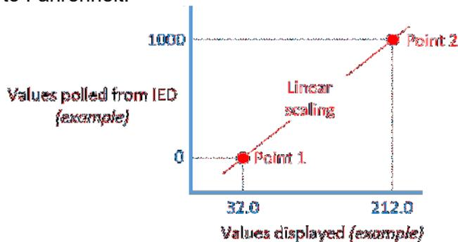
Some standard scaling calc types and example measurements have been created as part of the default page as shown below:
