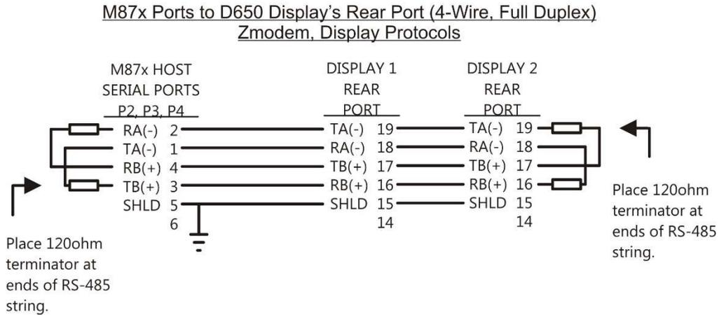
The rear port of the D650 and the Host port of the M87x must be set to RS-485, matching Baud rates and parity, and Display protocol.
