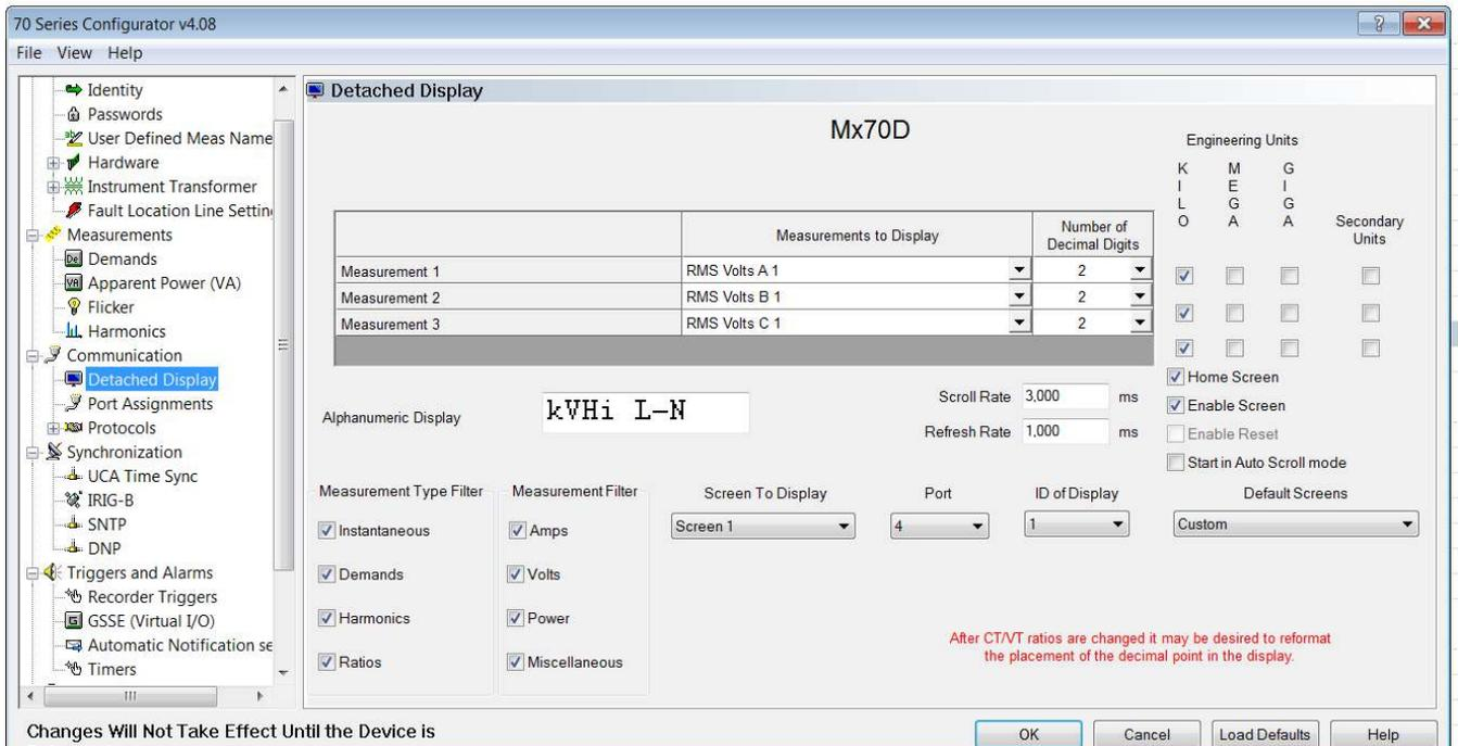
**Figure 8 – Configurator Communication/Detached Display Folder**
