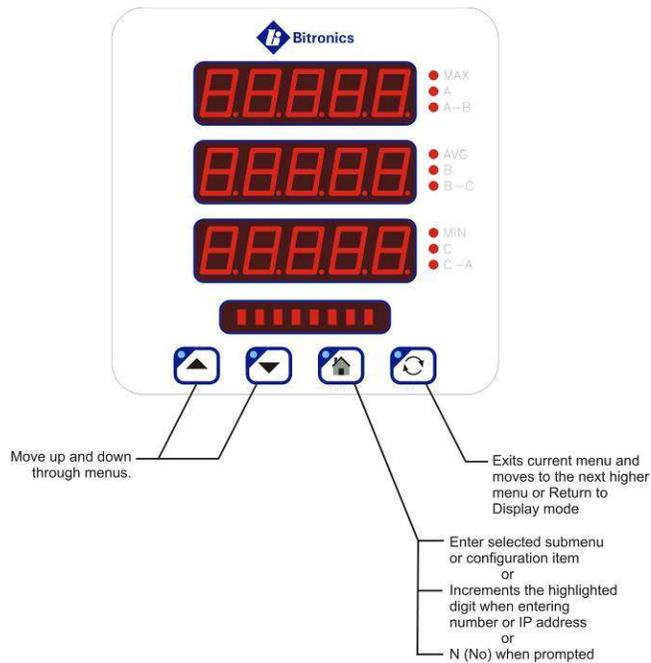
1. Setup mode is initiated upon pressing combination of Up Arrow and Exit
