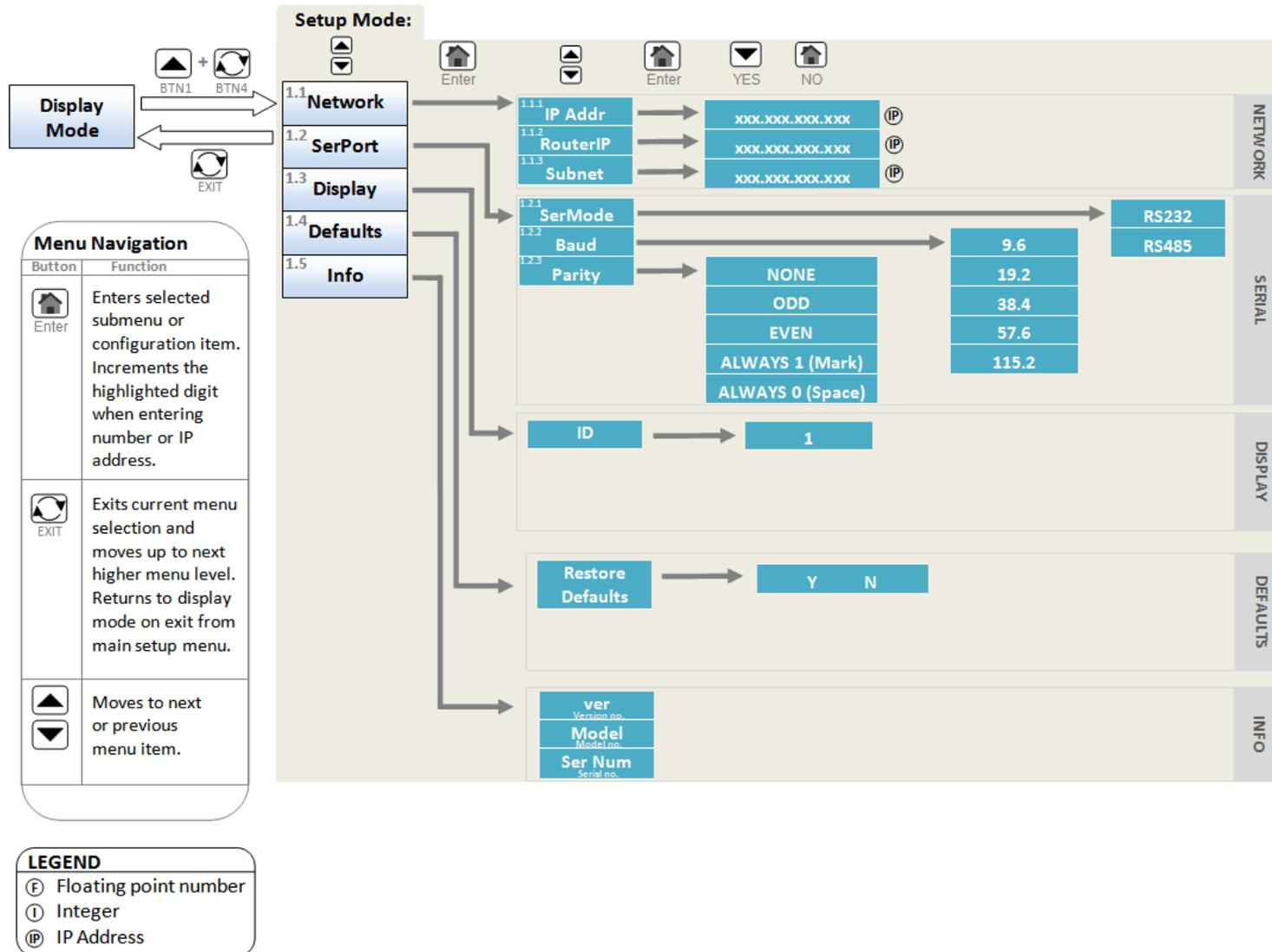
Figure 11 - D650 Front Panel Setup Menu
