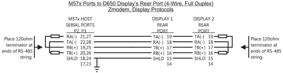
The rear port of the D650 and the Host port of the M57x must be set to RS-485, matching Baud rates and parity, and Display protocol.
