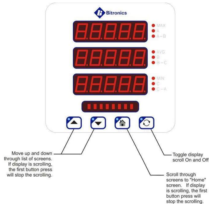
1. Pressing any button when the display is scrolling will end the scroll.
