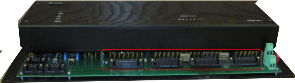
D20AD 32 AI with (4) DB25F connectors
