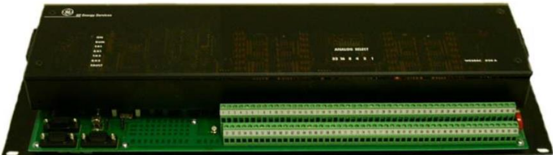
D20A 32 AI with compression terminals
