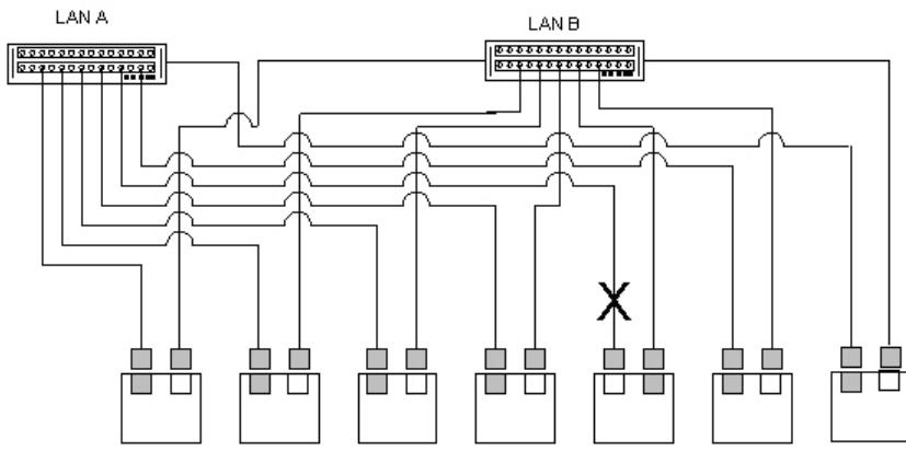
Figure 3 – Static Network Redundancy
