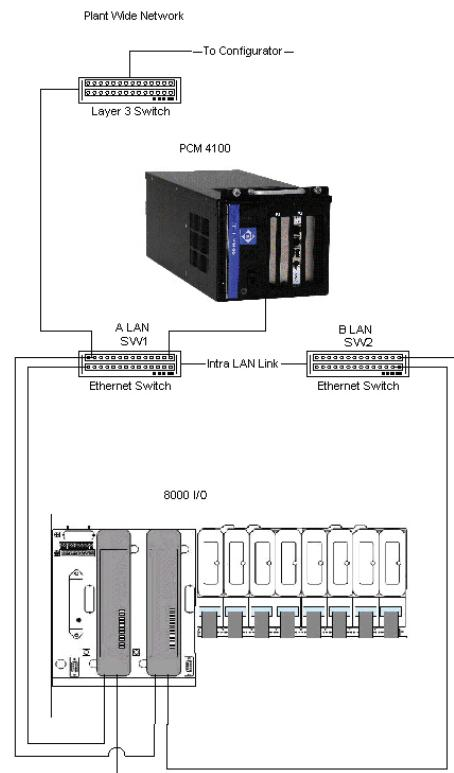
Figure 5 – Non-Redundant PCM Redundant EBIM Network Configuration
