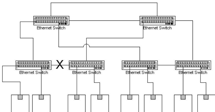
Figure 2 – Dynamic Network Redundancy<sup>[1]</sup>
