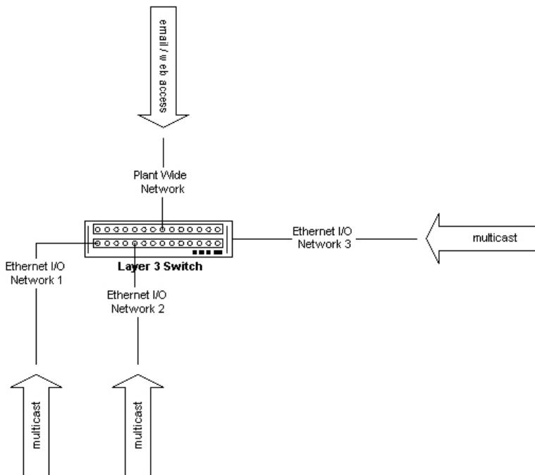
Figure 1 – Layer 3 Switch Configured to Isolate I/O Network
