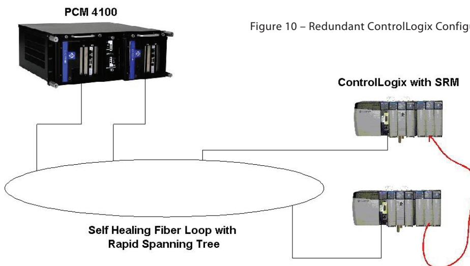
Figure 10 – Redundant ControlLogix Configuration
