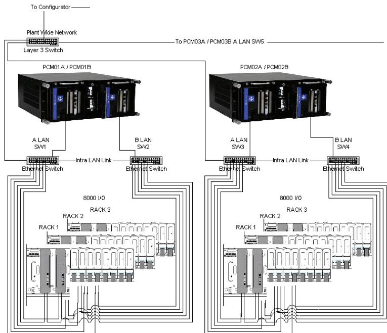
Figure 6 – Example Redundant Network Configuration
