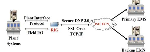
The OrionLX will serve as a Remote Intelligent Gateway for CAISO, providing encrypted data over secure TCP/IP to ISO EMS systems. Diagram excerpted from the CAISO paper "Remote Intelligent Gateway (RIG) Specification"
