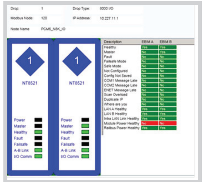
Figure 4 – 8000 I/O System Status Node Status Display
