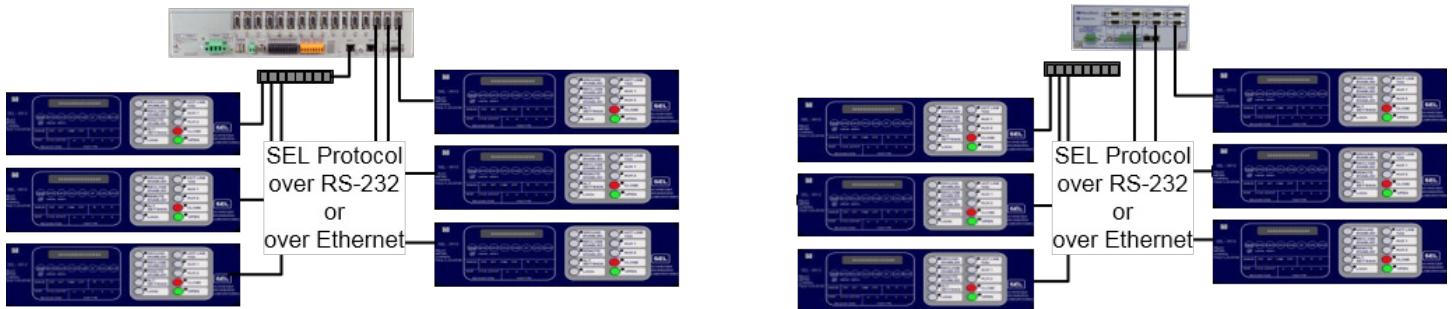
Figure 2: SEL settings are retrieved and backed up by the OrionLX or OrionLXm using SEL protocol over RS-232 or over Ethernet.
