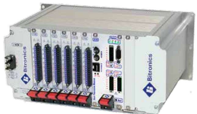
Bitronics 878 shown in wide chassis with standard V10 power supply, H12 host processor with E3 RJ45 plus 100FX Fiber Ethernet port, and six optional P30A digital I/O modules. The E1 Ethernet option with 100 Mbps RJ45 only is also available.
